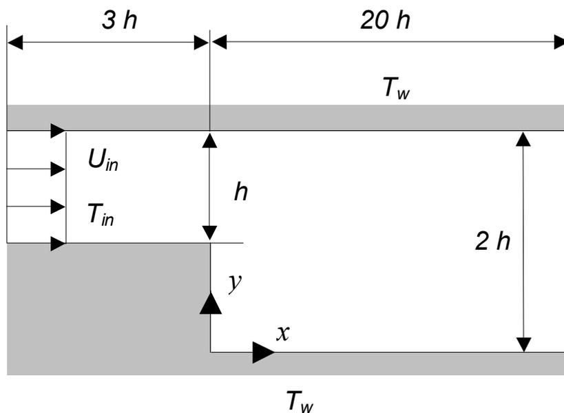
Figure 2. Sudden expansion geometry with its main dimensions.
