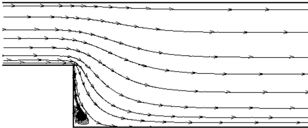
Figure 3. Streamlines at the expansion region for  $T_{in} = 423.0K$ .
