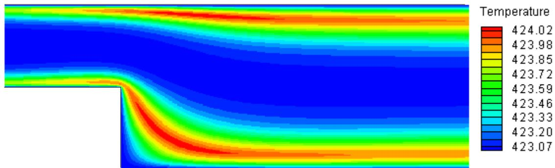
Figure 4. Temperature distribution for  $T_{in} = 423.0K$ .
