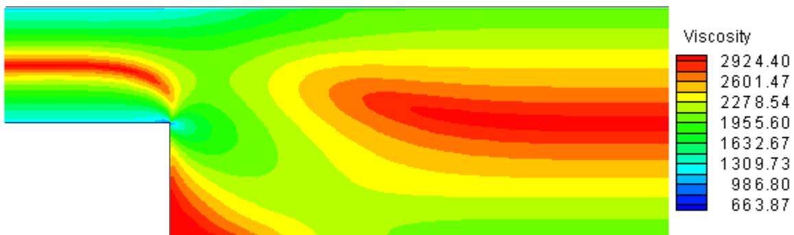
Figure 5. Viscosity distribution for  $T_{in} = 423.0K$ .
